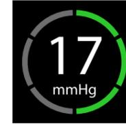
**Single mode:** Press the Measure button lightly to perform the measurement, **taking care not to shake the tonometer.** The tip of the probe should make contact with the central cornea. Six measurements should be made consecutively, green segments will be lit after every successful measurement. After each successful measurement, you will hear a short beep.
