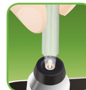
After loading the probe the tonometer will be ready for measurement when Play-symbol and active specie setting appears on the display.
