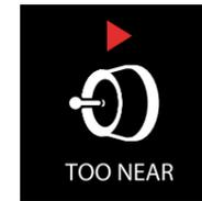
If there is an erroneous measurement, the tonometer will beep twice and display an error message. Press the Measure button to clear the error message. If several erroneous measurements appear, see error messages segment for additional information.
