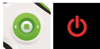
If you do not use the tonometer, it will switch off automatically after 3 minutes.
