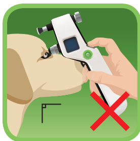
Incorrect alignment of the tonometer and red probe base light indication.
